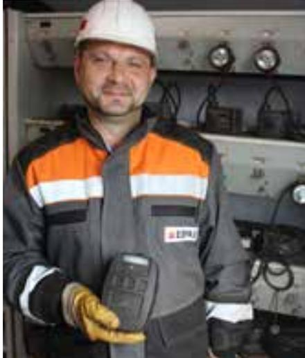
Lock-out systems are being installed to protect people from moving equipment and tunnelling faces at the Mezhegyugol mine and other EVRAZ mines. The main component of the STRATA Hazard Alert system is a magnetic field generator, which is installed on a piece of equipment and creates an electromagnetic field around it. Before entering the mine, employees receive a personal signalling device that detects these fields.
