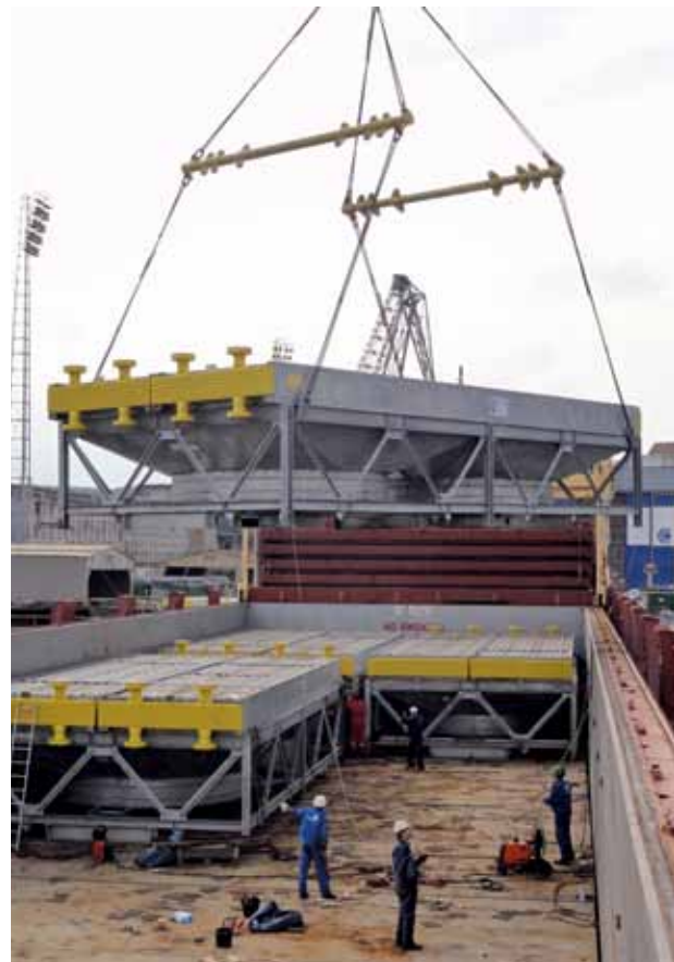
Air finned coolers being loaded for the Nord Stream gas compression station, Russia
