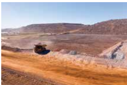
A haulage truck depositing material on the new leaching pad at Herradura
