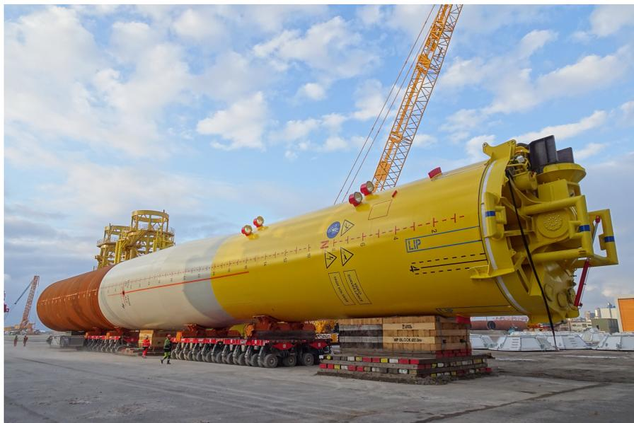
Picture: monopile for Hollandse Kust Zuid on SPMT
