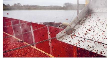
After harvesting, the cranberries are pumped onto a vibrating conveyor and loaded onto a truck.
