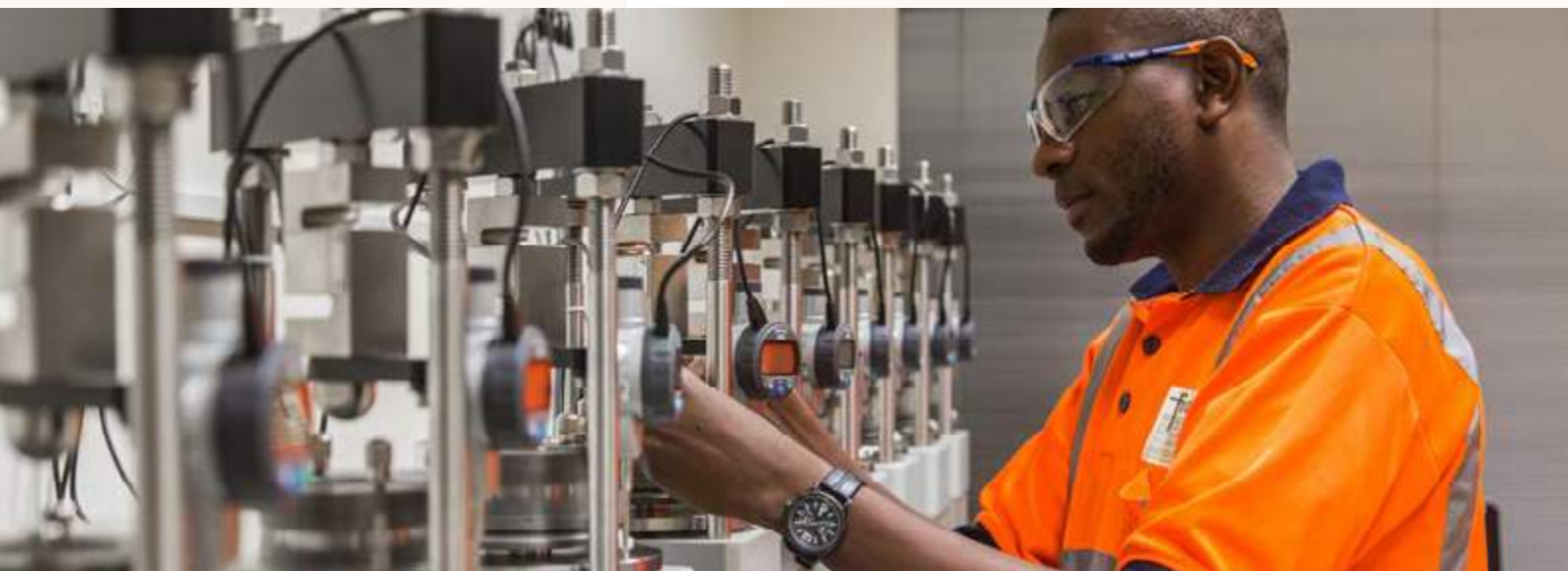
Oedometer test gives information on compressibility of soils, Luanda, Angola.
