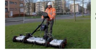
Ground Penetrating Radar (GPR) is a geophysical method that uses radar pulses to image the subsurface.
