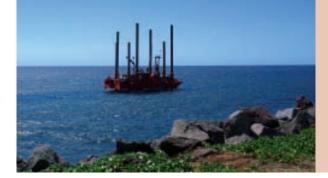
A Fugro Seacore jack-up platform taking samples at La Réunion.
