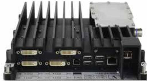
Our Nexxis RNA adapters support uncompressed streaming of desktop content (DVI, audio, USB) over the IP network, **enabling real-time interaction with remote servers or computers** – without dedicated video switches and without sacrificing image quality!
