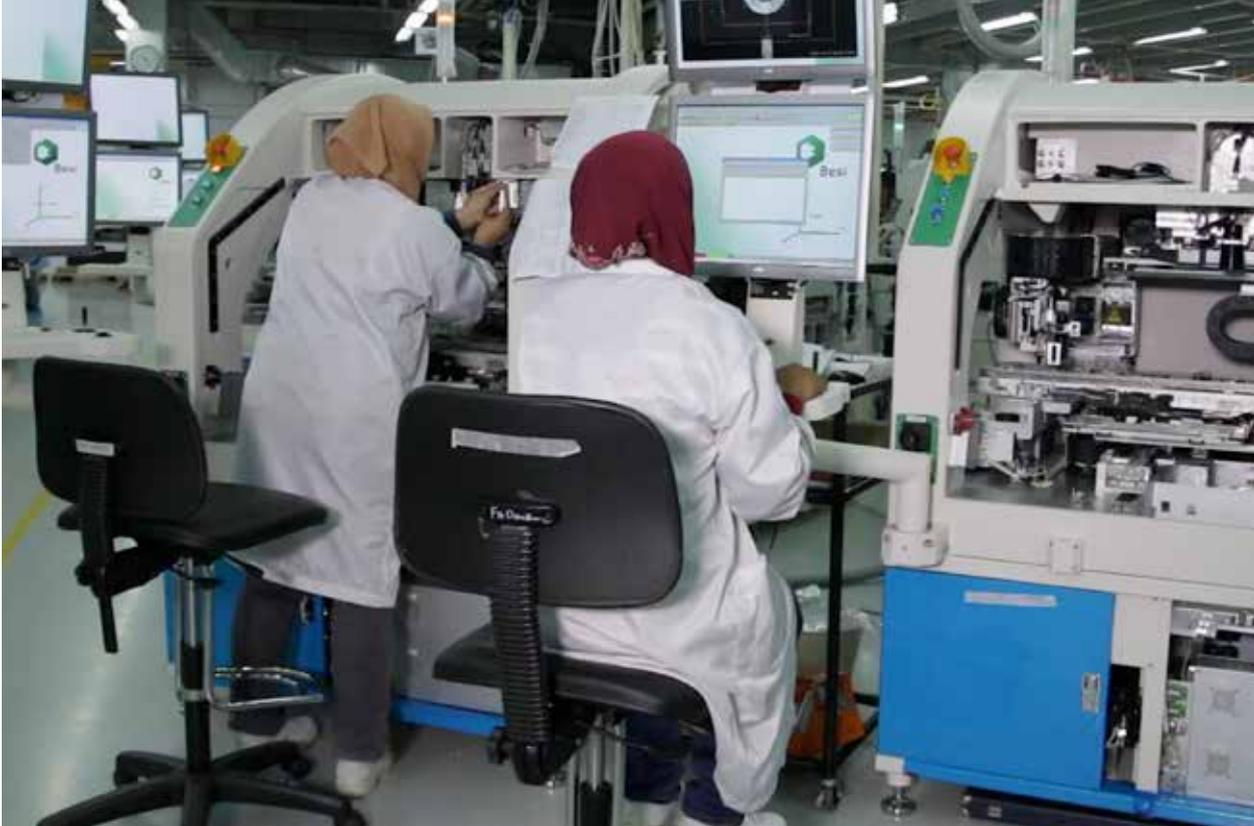
*Application engineers at Die Attach Besi APac, Malaysia, performing an internal system buy-off*
