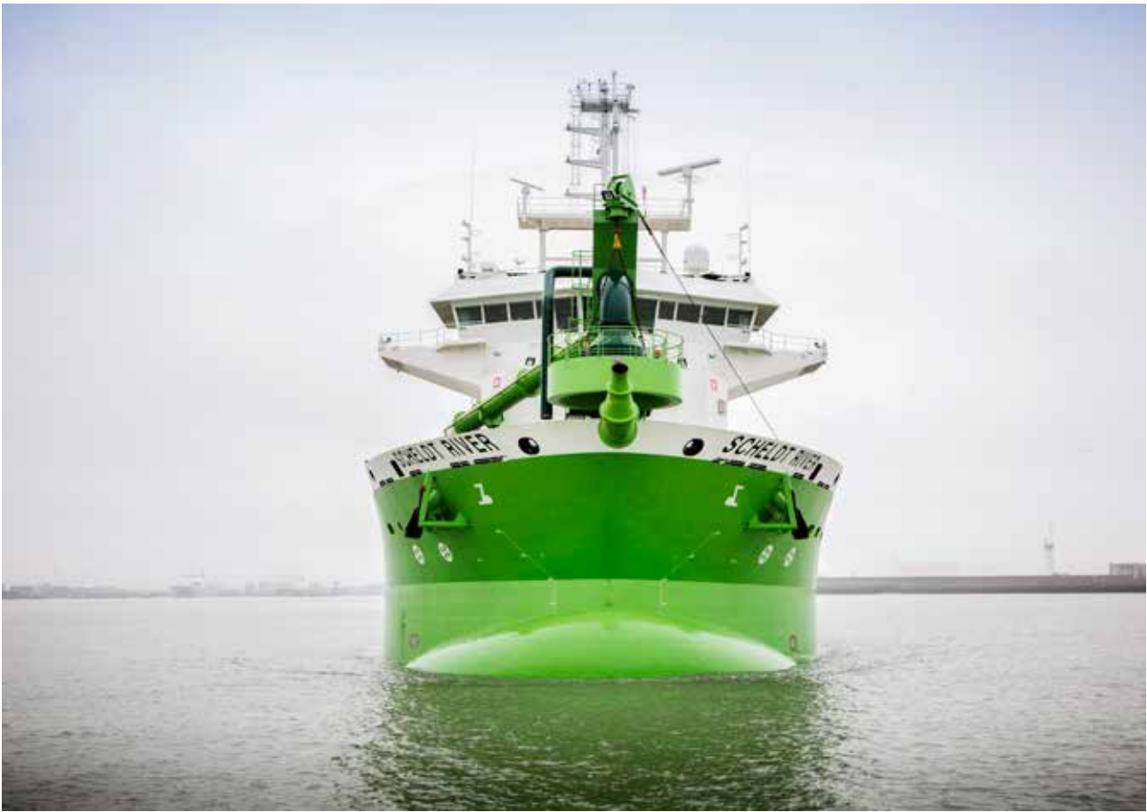
The new dual-fuel hopper 'Schedt River'
