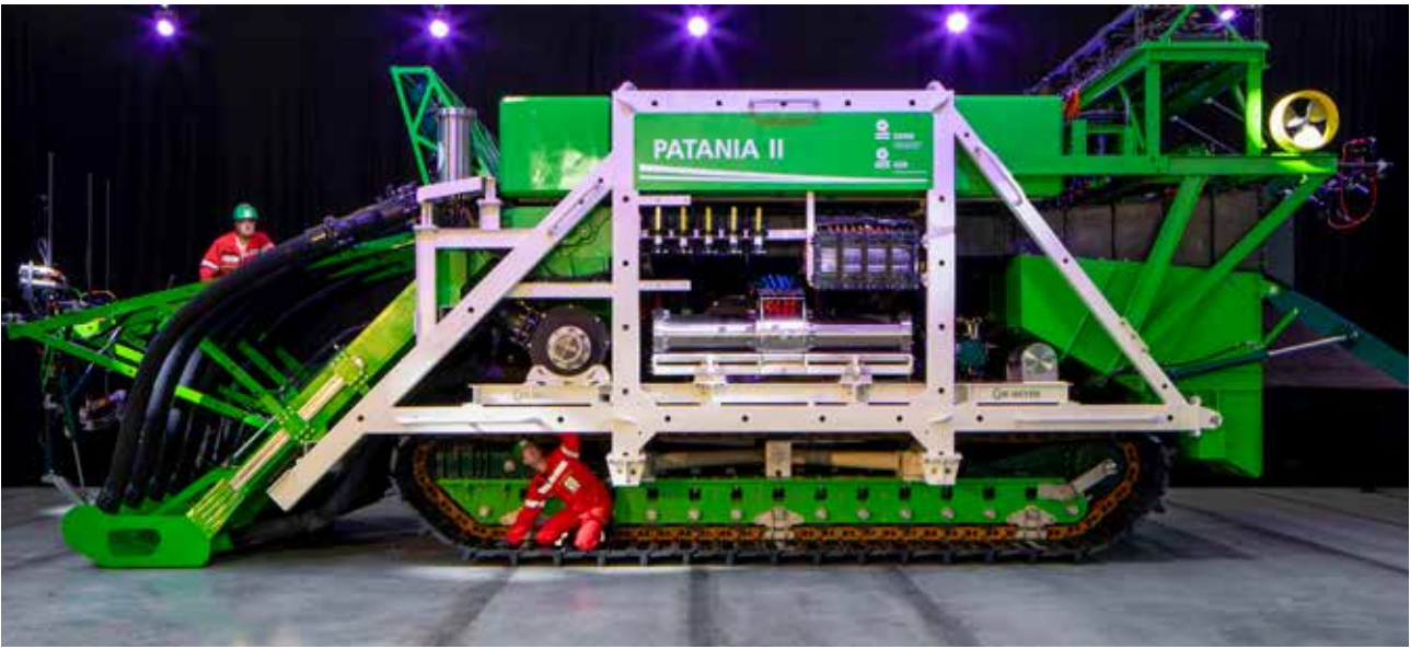
The nodule collector 'Patania II'
