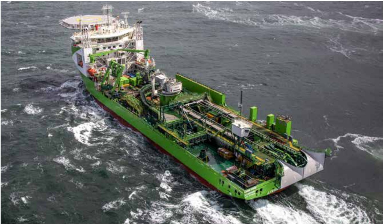
The dual-lane cable installation vessel 'Living Stone'
