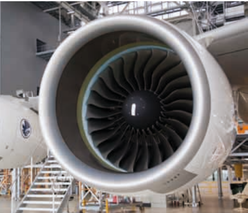
The A380 is equipped with four GP7200 engines. <<<
