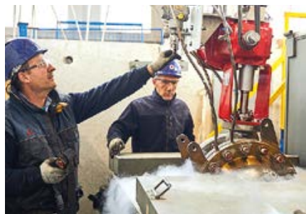
IMI Critical Engineering has world-class cryogenic testing facilities, for all classes of valves. Here butterfly valves are being lowered into the liquid nitrogen
