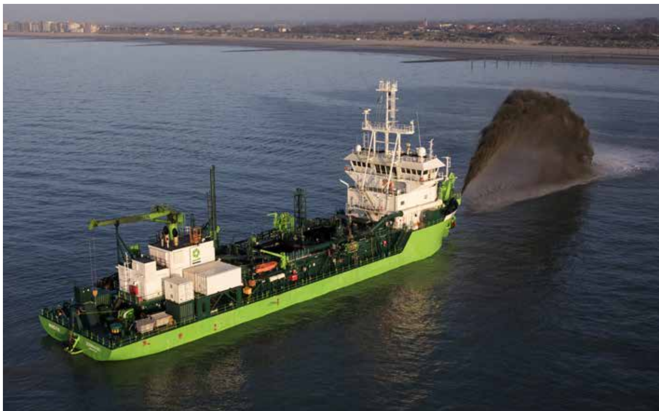
DEME - The Minerva is the first dredger in the world that can operate on LNG
