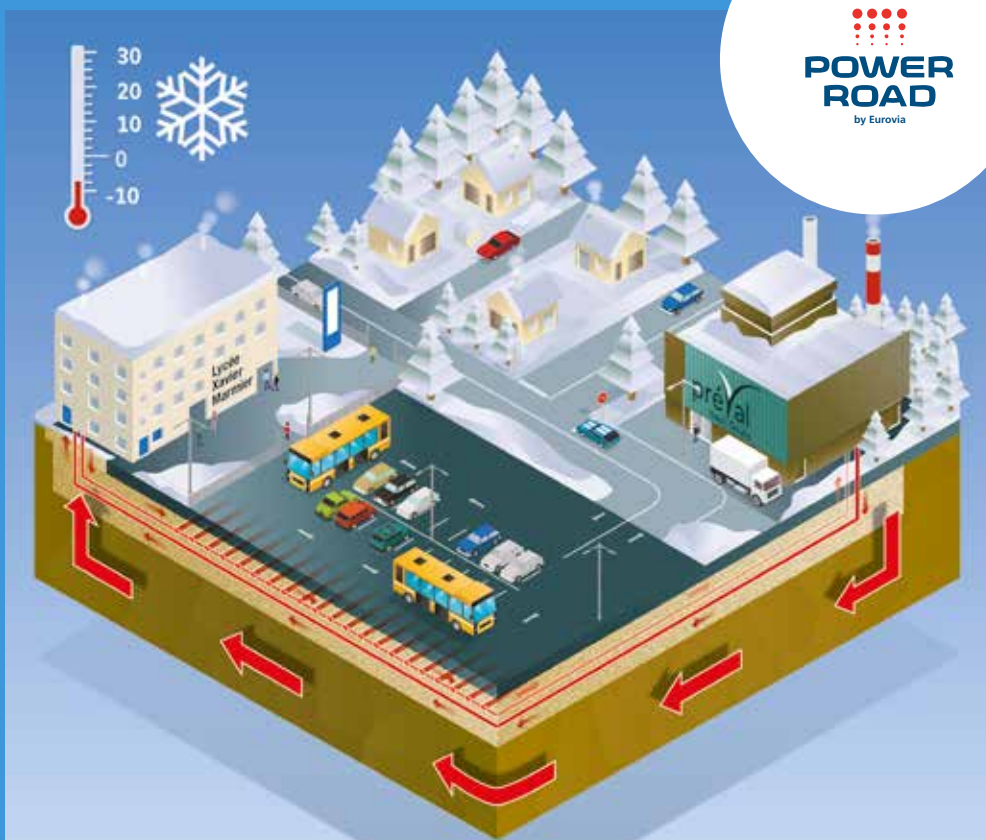
Installation of Power Road® in Becquerel square in Pontarlier, in eastern France. The source of energy to clear snow from the car park is the heat from household waste combustion at the energy-from-waste facility (Valopôle).
