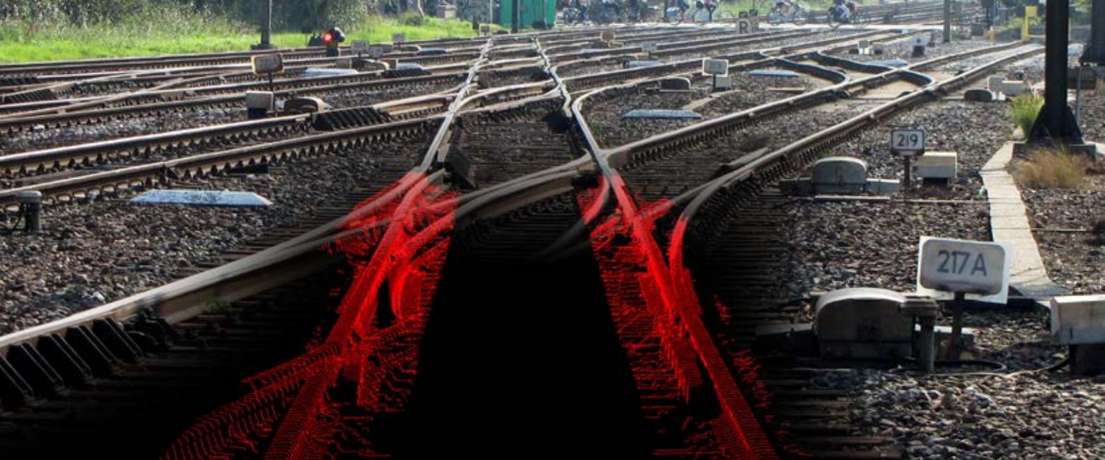
3D measurement of millimeters accurate track positions, to optimise rail safety and track management.
