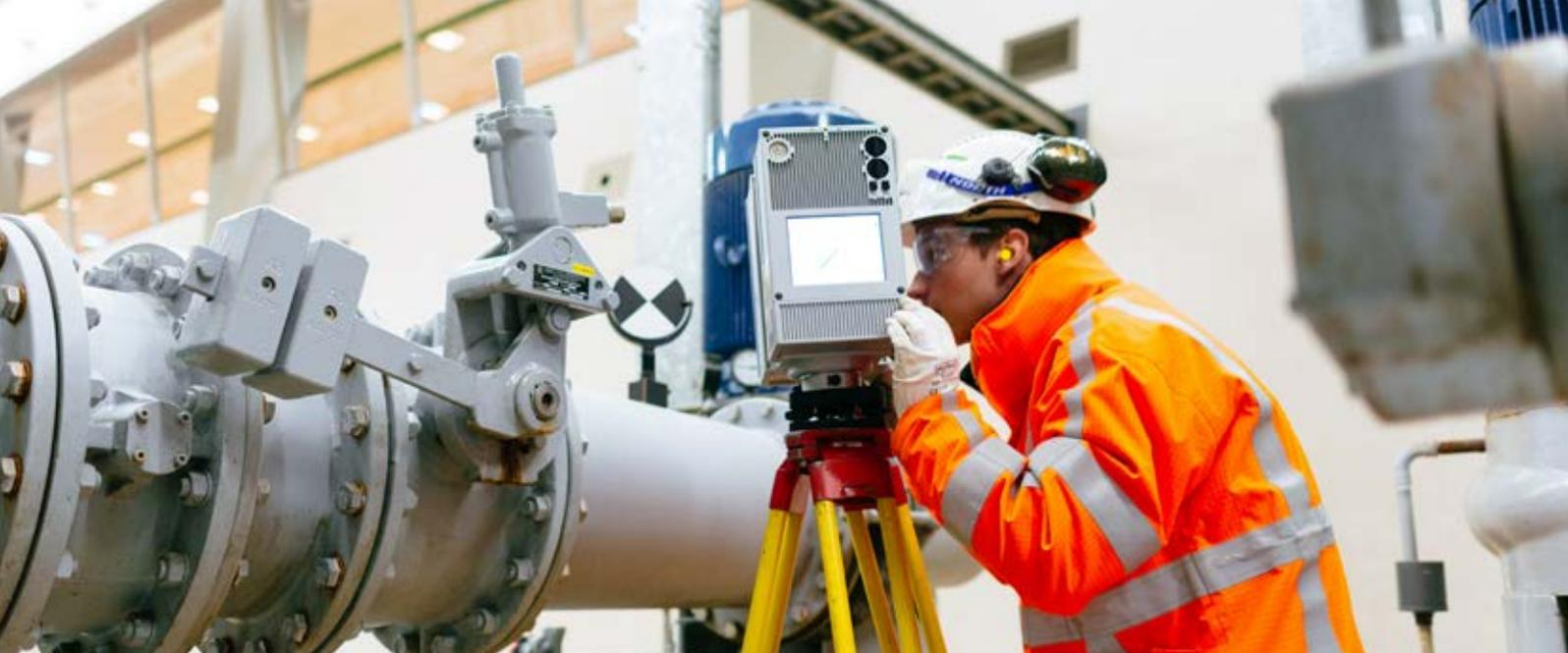
3D scanning of industrial installation, targeting efficient asset management.
