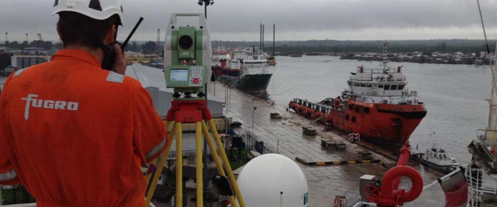
Calibration of vessels' instrumentation from quay side.
