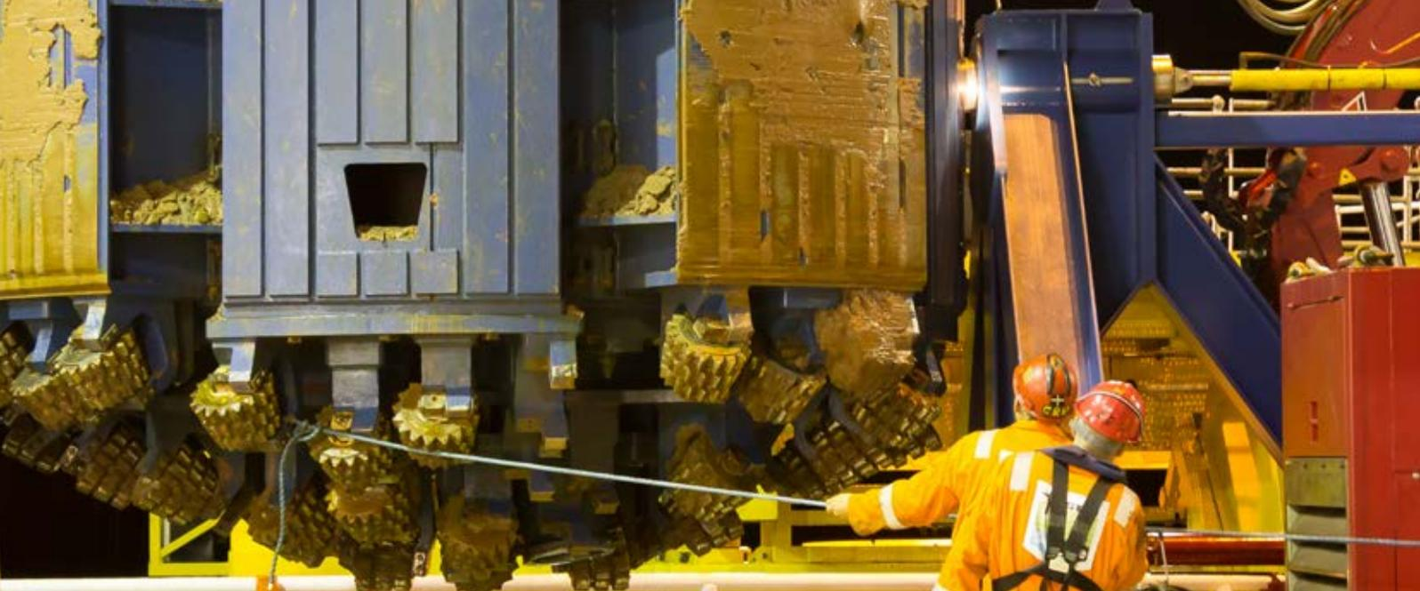
*Drilling of large diameter vertical shafts.*
