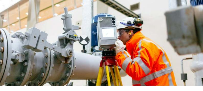
3D scanning of industrial installation, targeting efficient asset management.
