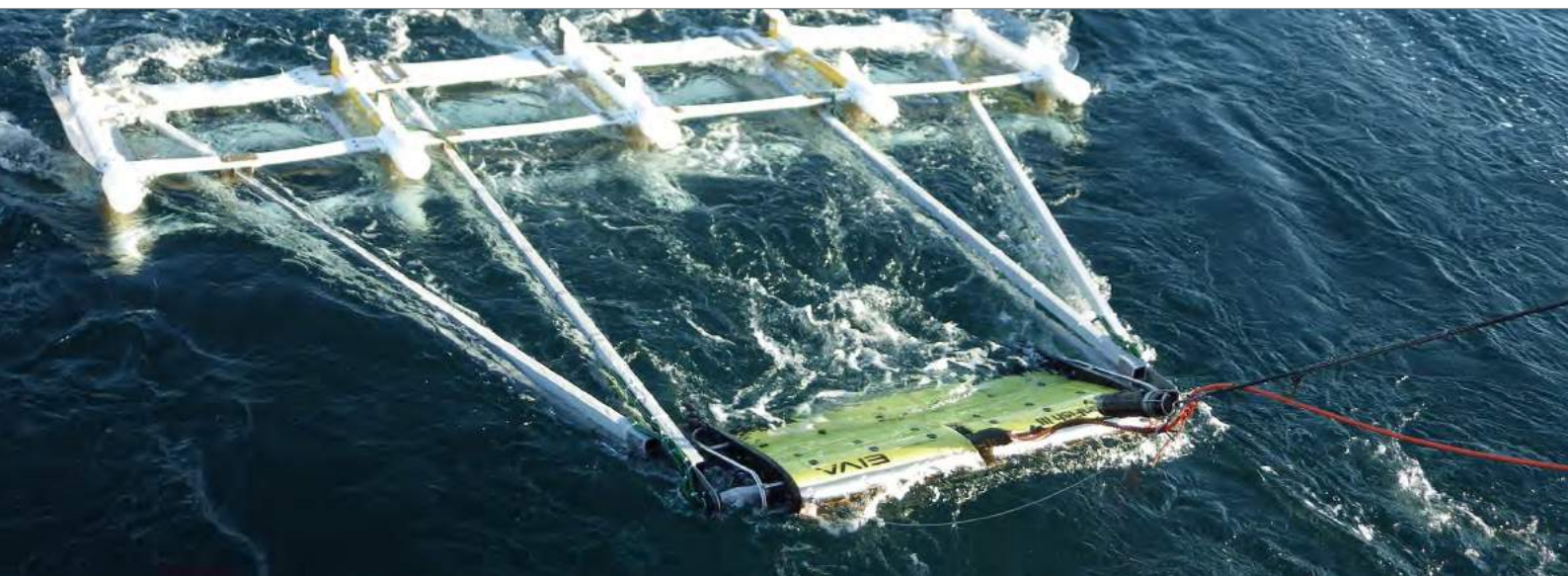
Fugro Geowing collects high resolution magnetic data, in order to detect unexploded bombs
