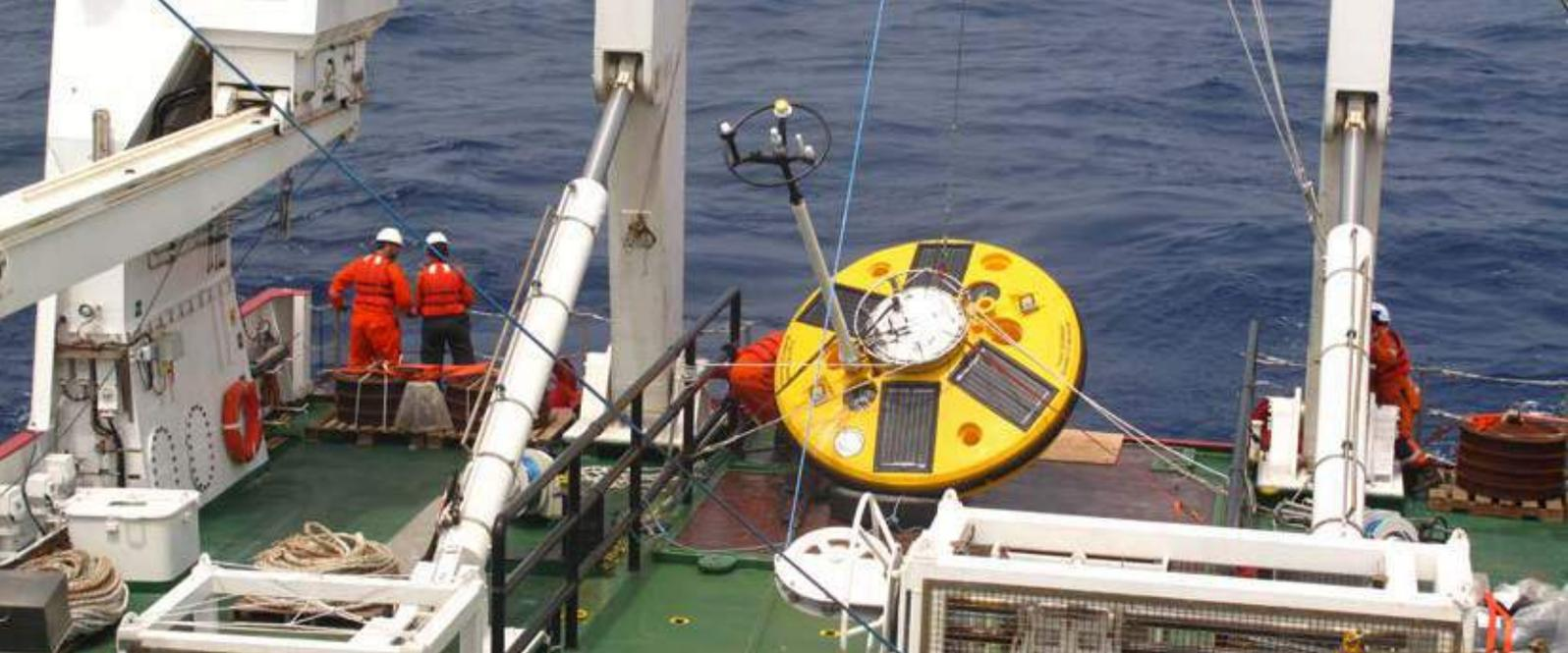
Wave scan buoy onboard survey vessel Fugro Brasilis.
