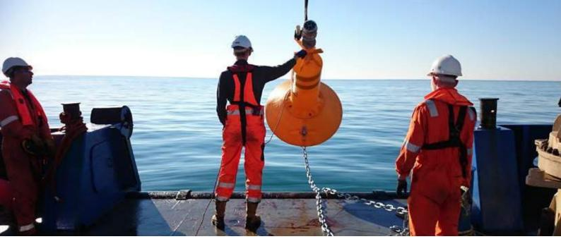
Deployment of buoy for measuring waves and water currents.
