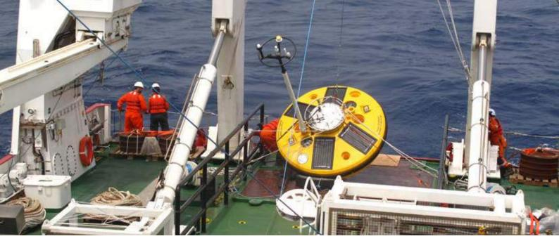
Wave scan buoy onboard survey vessel Fugro Brasilis.
