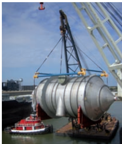
Unloading of a scrubber for a refinery in the USA
