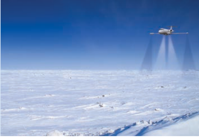
Artist's impression of Fugro Gulfstream-II jet aircraft equipped with GeoSAR sea ice mapping system in Arctic region.
