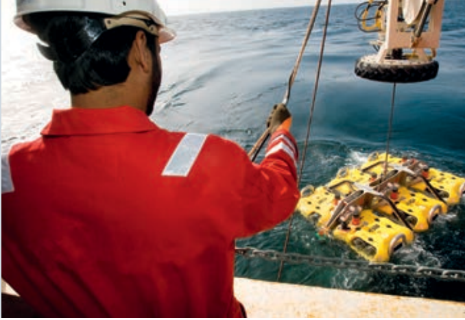
Caption: Ocean bottom nodes deployment, Middle East
