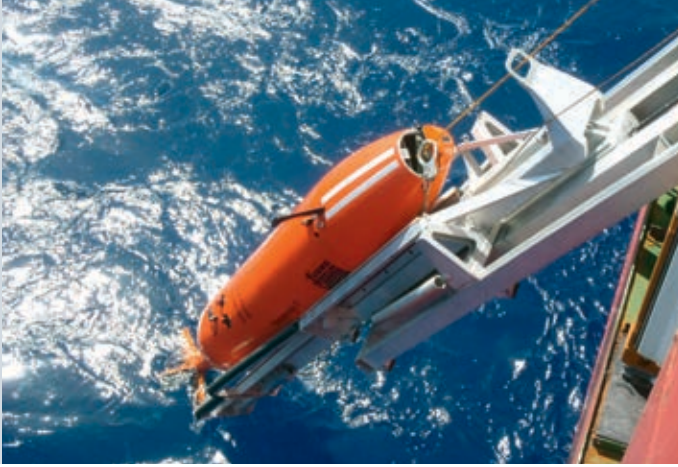
AUV deployment for seabed survey, Gulf of Mexico.
