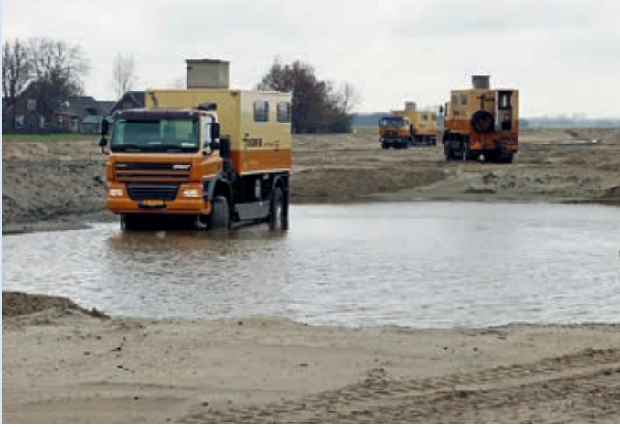
Fugro trucks performing cone penetration test, Delft-Schiedam, The Netherlands.
