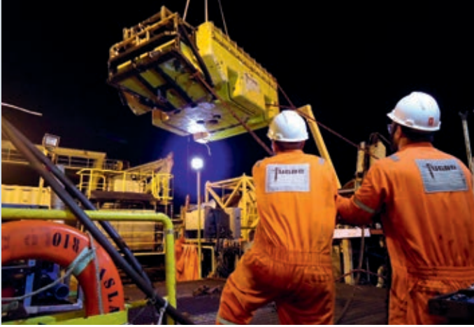
Recovery of a remotely operated vehicle (ROV) on board a ROV support vessel Island Spirit, Brazil.
