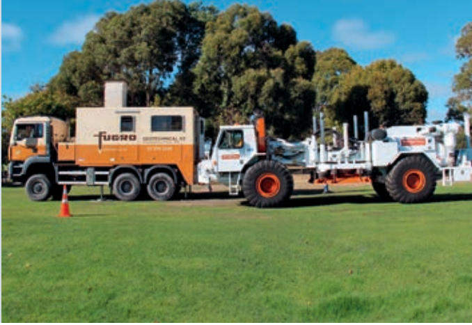
Fugro CPT truck collecting data for ground model analysis and design related to earthquake engineering, Christchurch, New Zealand.
