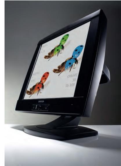
First ATC main display with replaceable LED backlights
