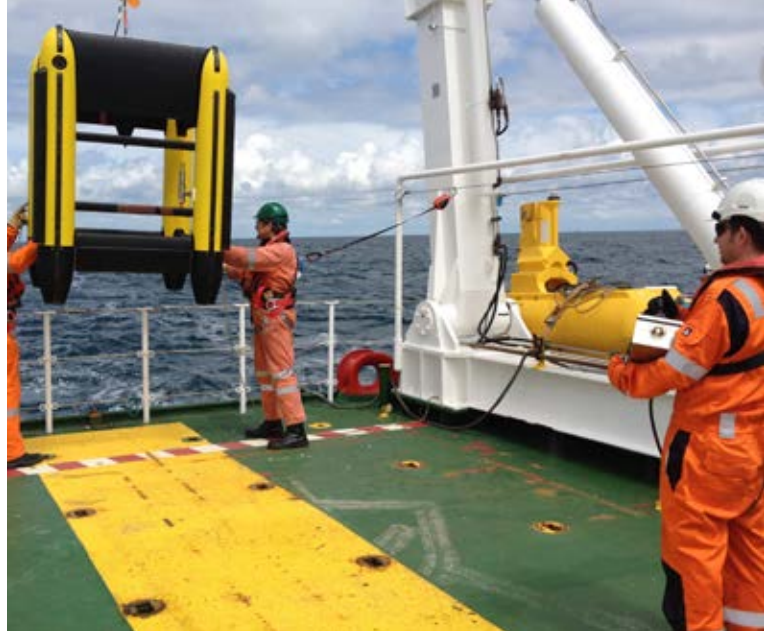
Launching a remotely operated towed vehicle for pipeline inspection operations, Southern North Sea UK Sector.
