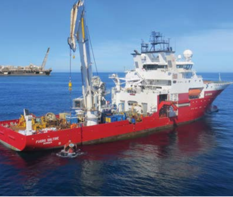
Deployment of thruster from ROV support vessel, Fugro Saltire.
