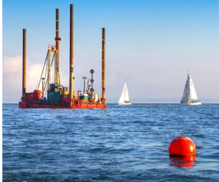
Fugro Seacore jack-up barge Coastal Explorer during site investigation in Cowes, United Kingdom.
