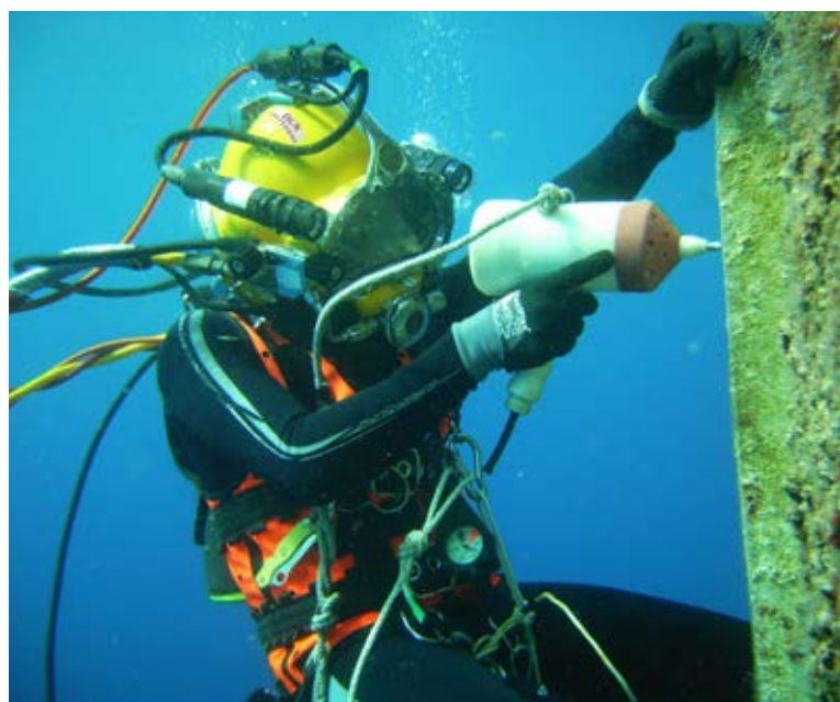
Diver testing the cathodic protection of an offshore platform, Middle East.
