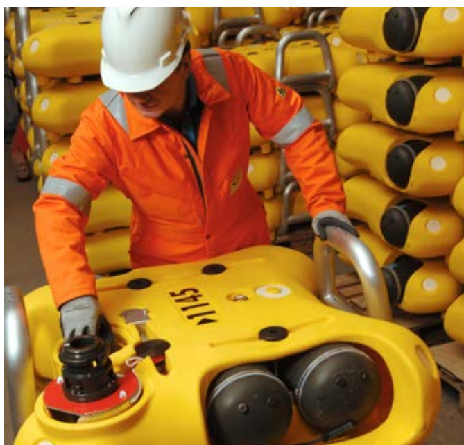
Preparing ocean bottom nodes before deployment.
