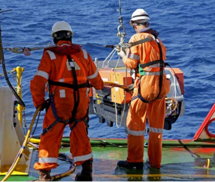
Deployment of deep tow scanner in search for the missing airplane MH370, Australia (source: ATSB; photo by ABIS, Chris Beerens, RAN).
