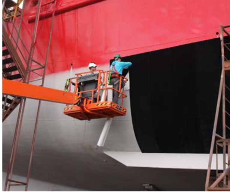
Vessel being outfitted with advanced hull coating, which should lead to lower fuel consumption.
