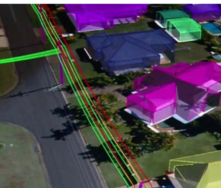
3D mapping of power lines, Australia, for asset management.
