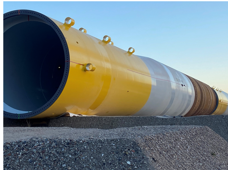
Picture: the diameter of a monopile refers to the diameter at the bottom. Towards the top of the monopile, the diameter reduces to 7.5-8.5 meters using cones to match the diameters of the tower or transition piece
