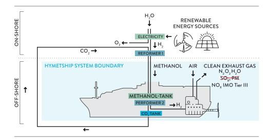
system for  ${\rm CO}_2$  and methanol as well as a hydrogen-fueled internal combustion engine into one system (Figure page 32).
