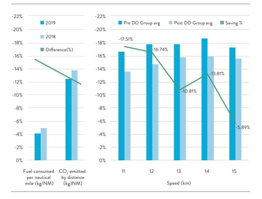
In 2019, the EXMAR Fully Pressurized fleet completed the second special survey dry dock. Maintenance works on the engines, hull and propeller performed during these technical stops, lead to a fuel efficiency increase as per following graphs.
