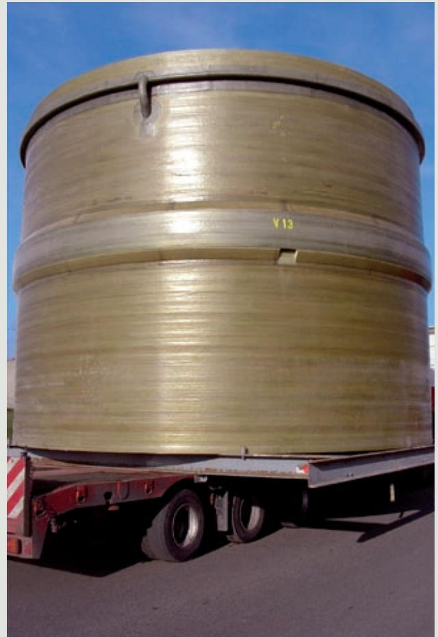
FRP elements for flue gas ducts, manufactured by the new subsidiary ACS ▶
