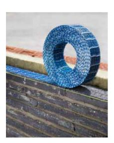
Murfor® Compact, Bekaert's high-performance masonry reinforcement is a sturdy mesh of high tensile strength steel cords, supplied on a roll for thin joint masonry and glued brickwork. The strong structure of the reinforcement controls cracks and strengthens masonry. This lightweight product is easy to handle and install. As the product can be cut to size on-site, there is almost no material loss.
