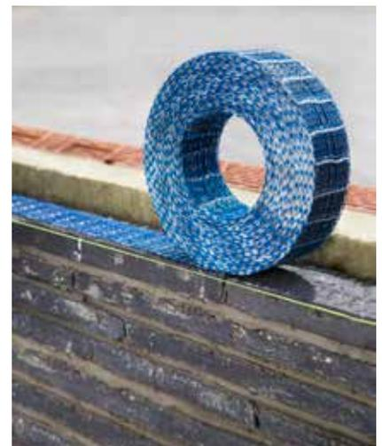
*Murfor® Compact, Bekaert's high-performance masonry reinforcement is a sturdy mesh of high tensile strength steel cords, supplied on a roll for thin joint masonry and glued brickwork. The strong structure of the reinforcement controls cracks and strengthens masonry. This lightweight product is easy to handle and install. As the product can be cut to size on-site, there is almost no material loss.*
