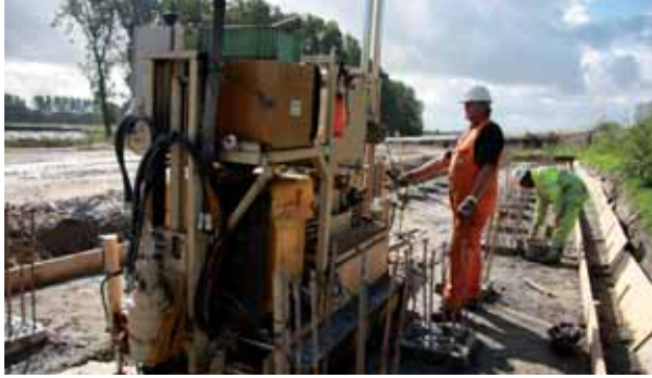
Cone Penetration Test with a mini-crawler, Weesp, The Netherlands.
